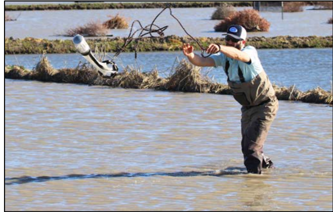
Zooplankton net used to measure amounts of fish food field in winter flooded rice fields.
